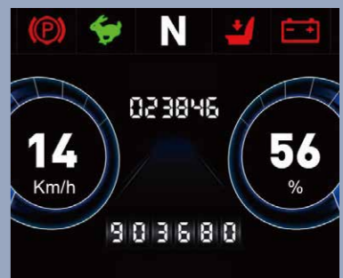
Multifunctional color screen instrument with graphical interface design is simple and intuitive for operator
