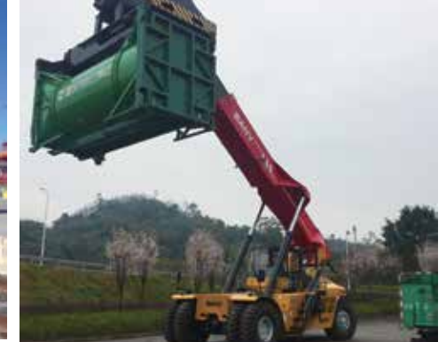
Sanitation Reach Stacker, Chongqing
